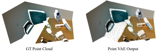
(a) Point VAE reconstruction. Even without diffusion, the VAE-reconstructed point cloud exhibits substantial noise, which fundamentally limits the quality attainable by latent diffusion models.
